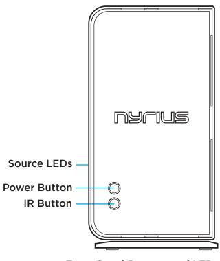
Front Panel Buttons and LEDs
