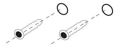
(4 )Place NAVS502 main holes over the protruding screws and slide down into positio
