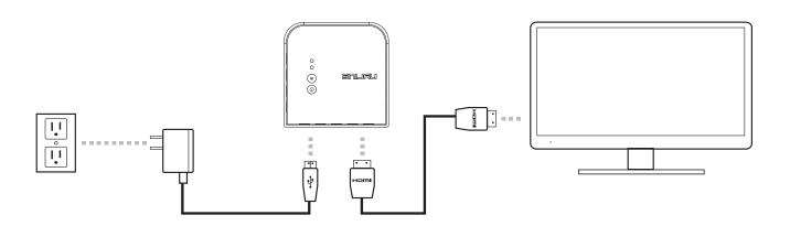
Connect the receiver's "HDMI OUT" to the HDTV's "HDMI IN" port.
