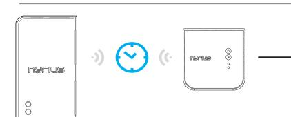
During the warm-up, the POWER LED will blink until connection between the TRANSMITTER and the RECEIVER is established. It will take 15 - 20 seconds for the system boot up successfully.
