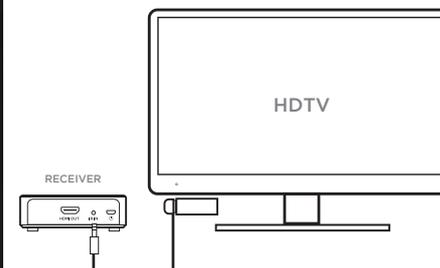
NOTE: Obstacles will decrease the distance of the IR extender. Transmitter and source devices connected to the Transmitter must all be in line of sight for IR control.
