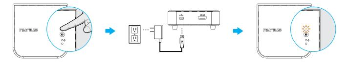
Plug the power adapter into the Transmitter. Press and hold down the pairing button.
