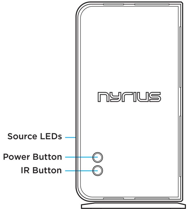
Front Panel Buttons and LEDs
