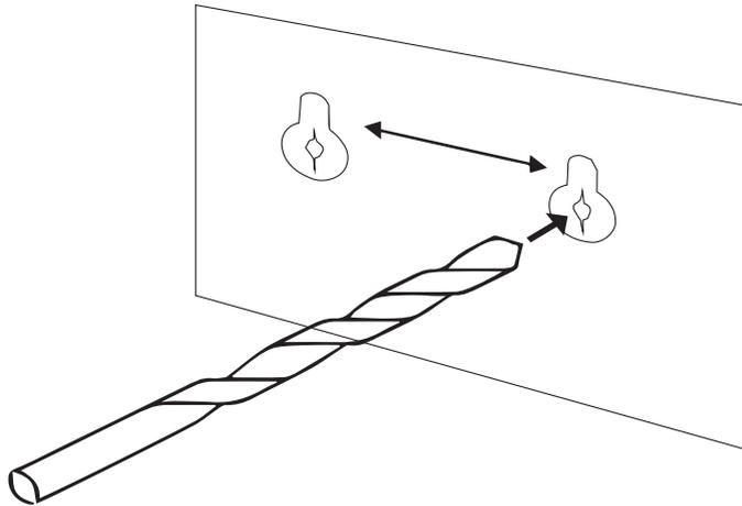
**(3) Insert two screws into the anchors. Leave 1/8" length for mounting the Transmitter or receiver.**
