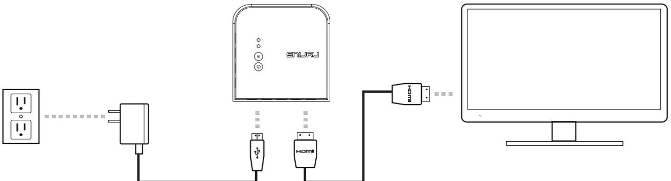
Connect the receiver's "HDMI OUT" to the HDTV's "HDMI IN" port.
