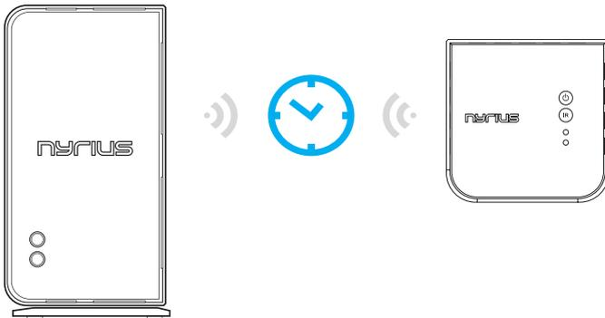
During the warm-up, the POWER LED will blink until connection between the TRANSMITTER and the RECEIVER is established. It will take 15 - 20 seconds for the system boot up successfully.
